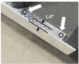
4. Lastly, drive (1) #10 x 1.5" Self Tapping Screw into the side of the Rocker Panel near the rear wheel well and the seam of the factory Rocker Panel. The screw placement should be equal distance between the top and bottom of the Rocker Panel.
